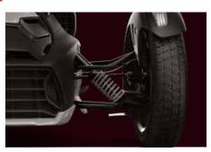
**KYB SUSPENSION:** Allows 1 inch extra suspension travel and adjustability on the rear which provides four different compression settings to optimize your ride.
